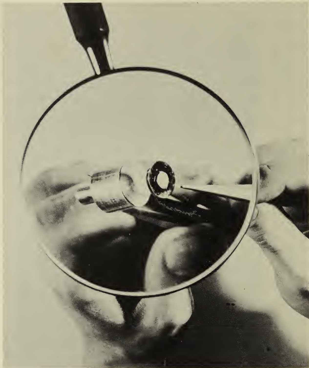
Fig. 37. A magnified view of an atomic cell in its final stages of assembly. Here the transistor-like junction is being put in place. The position of this junction is shown in Fig. 35. (Courtesy Radio Corporation of America)
